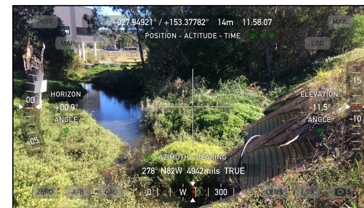
EXAMPLE OF THEODOLITE PHOTO SHOWING BEARING AND LOCATION
